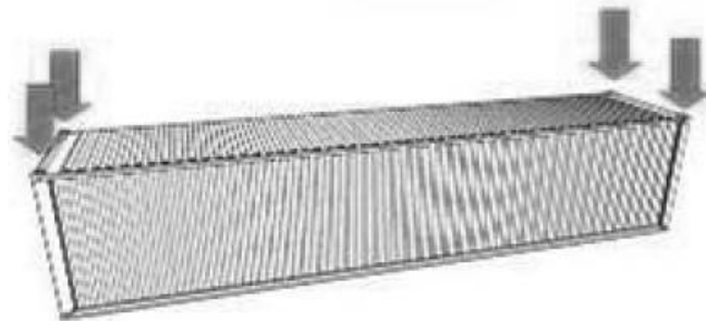
Figure 2.30. Transfer of vertical loads in containers (Anagal & Dhongde, 2017)
